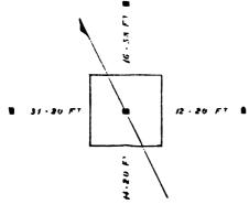
The pillar is solid, and raised about 4 feet above the summit of the hill. Four marks have been engraved on the rocks around, at the distances indicated in the sketch, and in such positions that the diagonals of the quadrilateral intersect each other over the station mark. The azimuth of the village of Shá-Kot is 252° 29', and distance ·7 mile.
